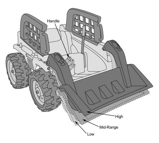
**IMPORTANT!** The bucket is designed to automatically drop to its lowest position with a load that exceeds 10 lbs. **Do not** modify the bucket to defeat this safety feature.
